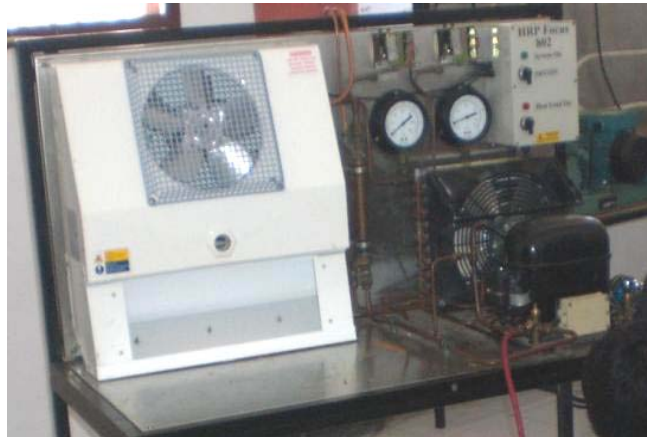
Gambar 4. Unit Pengujian Mesin Refrigerasi model HRP focus 802
